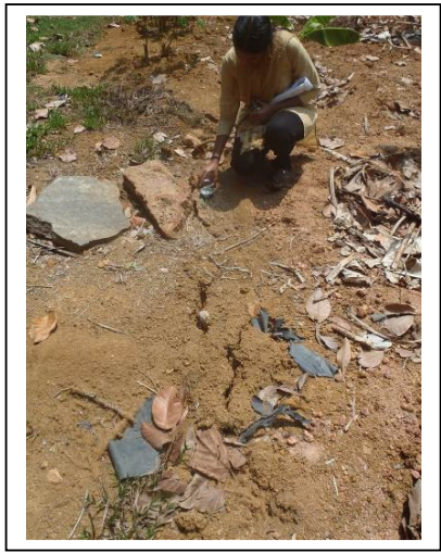
Figure 7: Measuring strike of ground fractures developed
