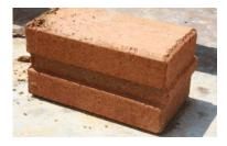
Figure 10-1: Interlocking mud block
