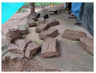
Figure 3-6: Making of mud bricks
