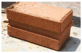
Figure 9-13: Interlocking mud block
