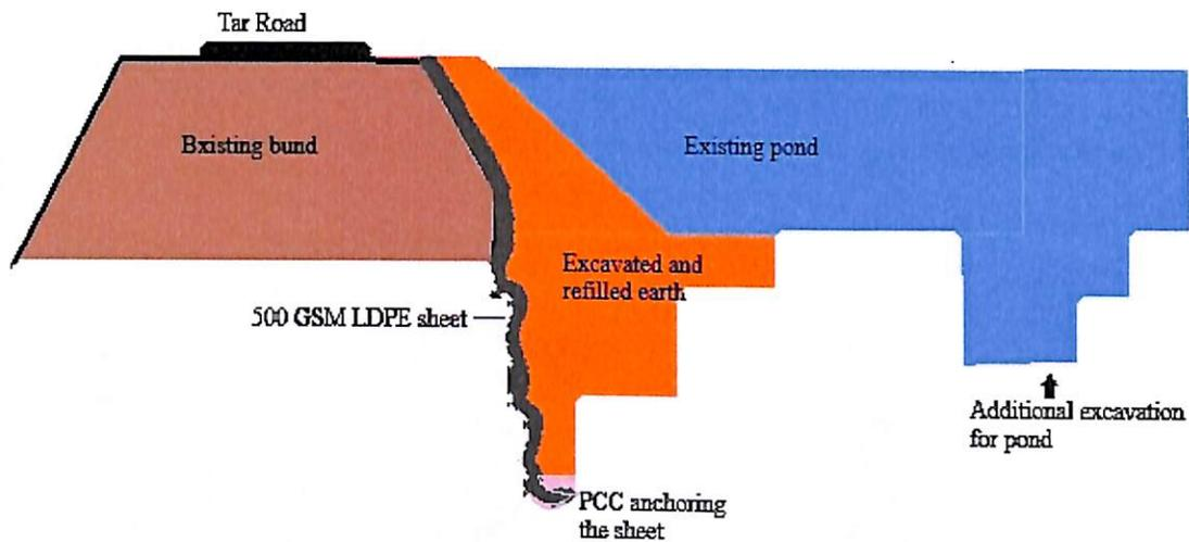
**Schematic section of the Sub-Surface dyke**
