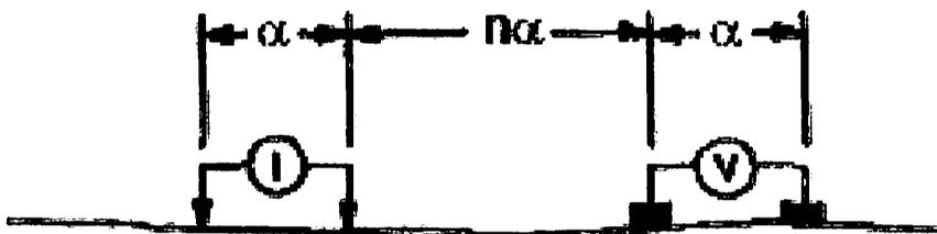
Figure 11c: Dipole - Dipole configuration
