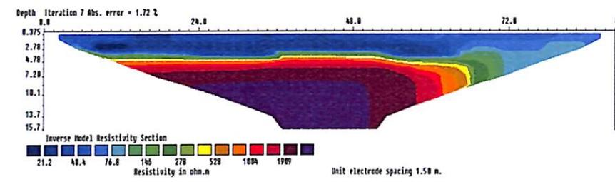
Figure: 14 2D images in different arrays at a separation of 2.5 and 1.5 m. Note the high resistance layer at a depth of 5m-7m
