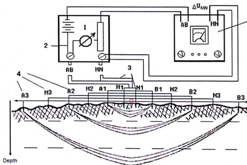
a) A, B Current Electrodes; b) M, N Potential Electrodes, c) O is Mid-point
