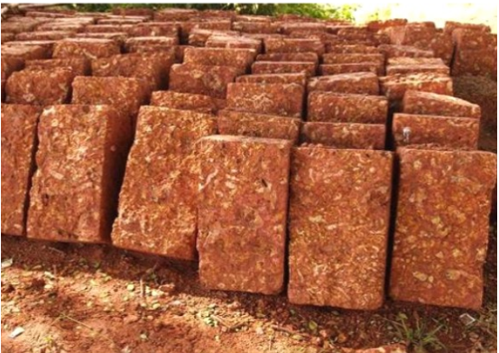
Figure 2-2: Prevalent Laterite Block used in housing construction
