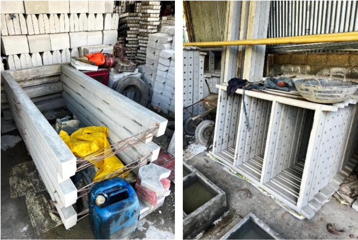
Figure 2-4: Precast concrete door and window frames manufacturing unit in Meppadi Panchayat
