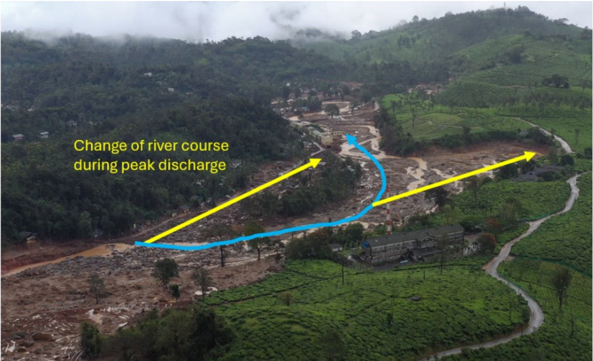
Figure 1-20: Bank breach point and deposition of saltation load and bed load on the left bank of Padavettipuzha along Chooralmala School Road marked with yellow arrow (Maneesha, 2024)
