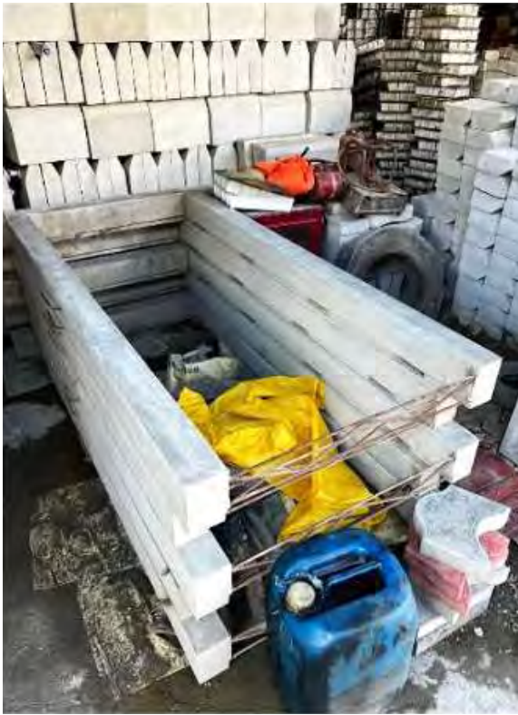
Figure 2-4: Precast concrete door and window frames manufacturing unit in Meppadi Panchayat
