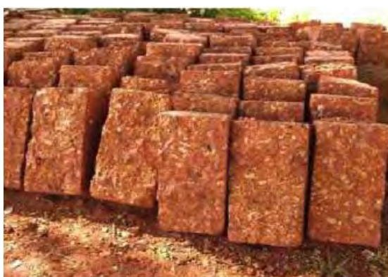
Figure 2-2: Prevalent Laterite Block used in housing construction
