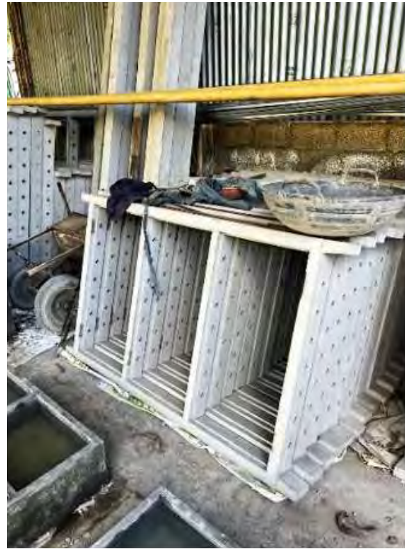
Figure 2-4: Precast concrete door and window frames manufacturing unit in Meppadi Panchayat
