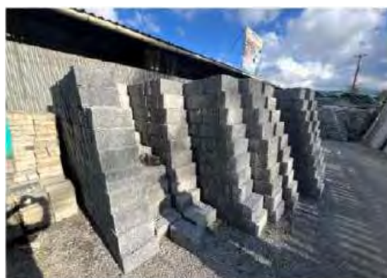
Figure 2-3: Solid concrete blocks used in practice in Meppadi Panchayat
